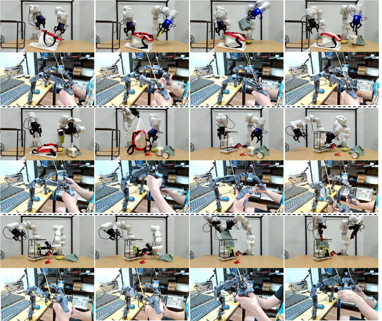
Fig. 5: Overview of the leader–follower arm teleoperation workflow for the household kitchen–tidying task, showing the five sequential subtasks: (1) item unpacking, (2) shelf organization, (3) towel folding, (4) towel placement, and (5) clamp attachment.
